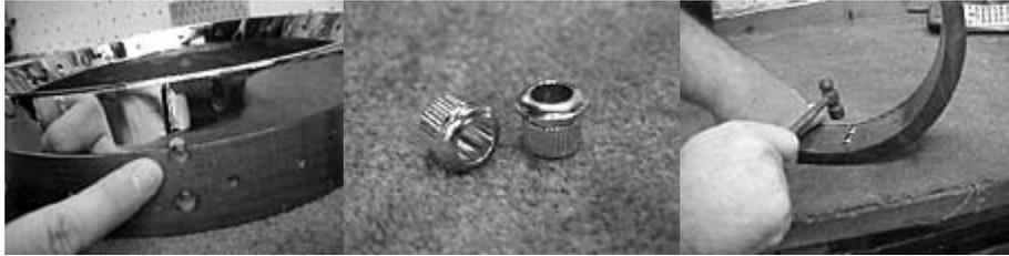
Align the tone ring onto the wood lining it up with the two holes that were already drilled in the wood rim. If the hole in the tone ring doesn't match perfectly, that is okay. Locate the inserts and install them with a light hammer.
