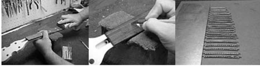
Using a wooden sanding block sand the fingerboard lightly with 220 paper. Then, using the back of a small, thin blade (I like the X-Acto knife) carefully clean out any glue or debris that may be in the fret slots. Line up the frets from the shortest to the longest using a straightedge as a guide.
