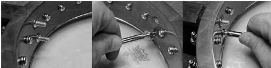
Slip the neck into place by guiding the lag screws through the holes where the inserts were placed. Start installing the top rod (on the bottom here because the banjo is upside down) The top rod has the small male threads on one end and is shorter than the bottom rod. Place the washer and the nut over the male threads then guide it through the hole as shown and attach the other end of the rod to the top lag screw as shown.
