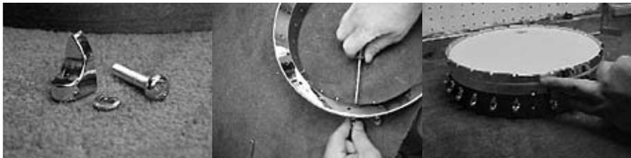
Locate the shoe brackets, screws and washers (there are 24 of each) and install them pointy side up. Take care not to over tighten. Place the head onto the pot assembly and align the center of the tension hoop notch over the two holes in which the inserts were installed.
