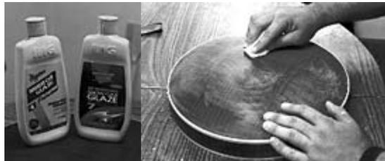
After the wet sanding is complete, and the entire finished surface is completely dulled, you will need to polish the finished surfaces. You will need 1 bottle of "Meguiar's Mirror Glaze #4" and 1 bottle of "Meguiar's Mirror Glaze #7". These are available through most automotive supply stores, or you can purchase them through Stewart MacDonalds Guitar Shop Supply.
