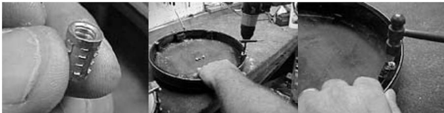
Locate the inserts, drill out the holes to a depth that is slightly more than is needed for the insert to seat. Drill the holes to the exact size of the outside diameter of the insert. Hammer the inserts into the rim of the resonator until they are flush.
