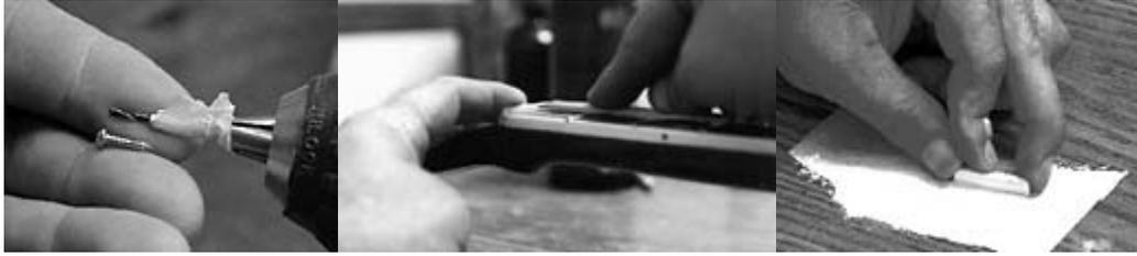
Use a piece of masking tape on the 1/16" drill bit used for pre drilling the holes for the screws used to fasten the headstock machines. This will help insure you don't drill through the peghead.
