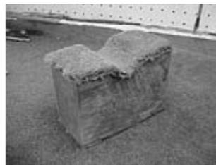
This is the neck block I use while assembling this banjo kit. It is made from a scrap piece of wood and has low pile carpet glued to it. The cut out for the neck needs to be a little larger than the size of the banjo neck. Make this or have a bag of buckshot standing by before you begin the assembly of the kit.
