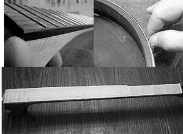
Using a safety razor blade carefully scrape away stain from the binding. Work carefully as scratches left by the blade will show in the finish. Tape off the fingerboard leaving a little space at the end of the frets on either side. We will scrape this away later. Put a piece of tape on the truss rod inside the opening, too.
